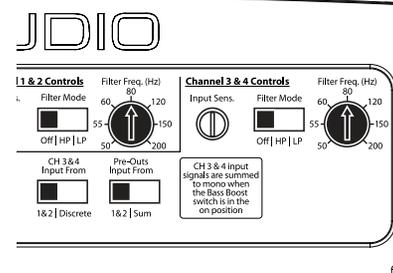
1) “Filter Mode” Control: The G4500 employs a 12dB per octave filter for each pair of channels (one filter for channels 1&2 and another filter for channels 3&4). Each of these filters can be configured independently into one of two filter types or defeated completely by way of the three-position “Filter Mode” switches:
